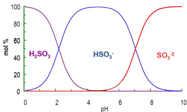
**Figure 2:** Equilibrium diagram of dissolved sulfite species is shown.<sup>40</sup>
